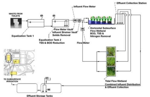
Fig. 3: Living Machine flow diagram
