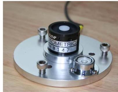
Fig. 8: LI-COR photometric sensor
