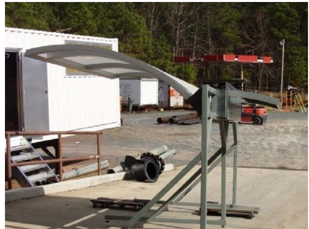
Fig. 7. Interior and exterior light shelf mock-up
