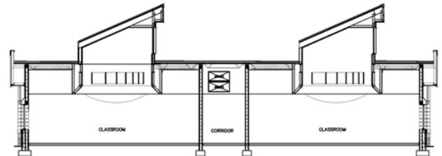
Fig. 7: Daylighting with south facing monitors
