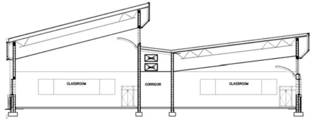
Fig. 6: Daylighting with no underfloor system
