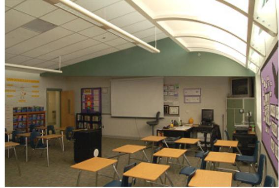
Fig. 13: Linear architectural shading element for AV equipment in a side-lit classroom with interior light shelf
