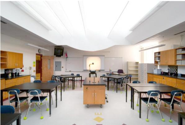
Fig. 12: Curved architectural shading element & splayed soffit design in a classroom with roof monitor
