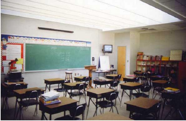
Fig. 11: Unwanted contrast at ceilings & AV location
