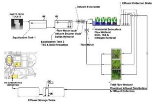
Fig. 3: Living Machine flow diagram
