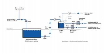
Fig. 2: Rainwater collection flow diagram
