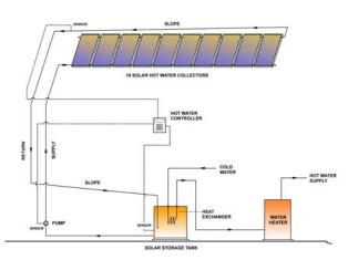
Fig. 9 Solar hot water schematic diagram
