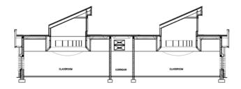
Fig. 7: Daylighting with south facing monitors
